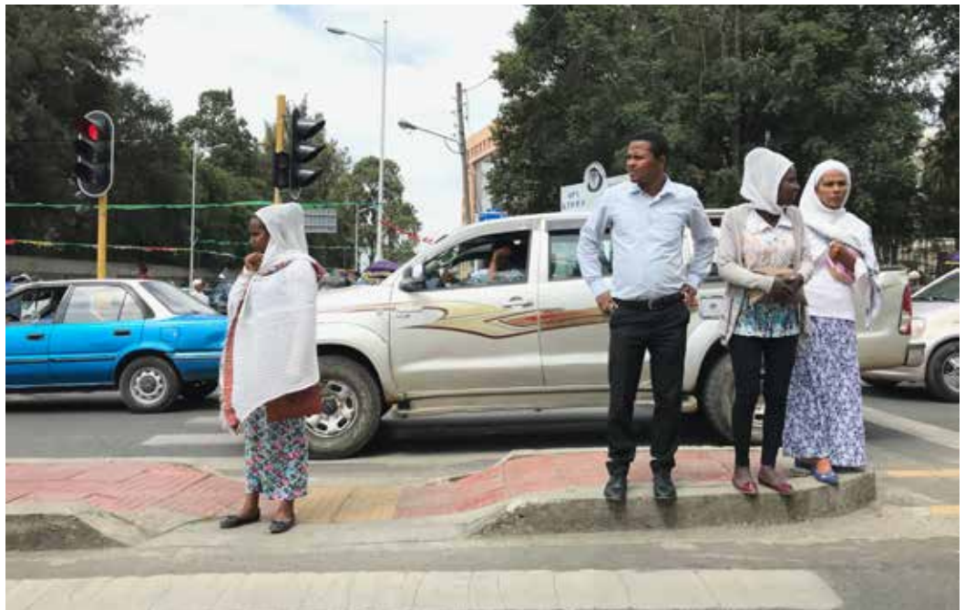
Figure 52. Medians offer a space for pedestrians to wait between streams of traffic.
