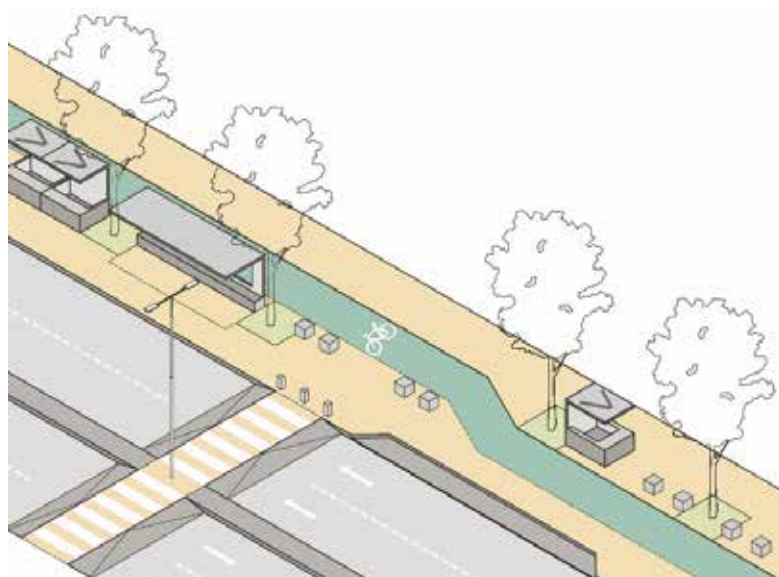
Figure 42. Shift cycle tracks behind bus stops to create sufficient waiting area for passengers.
