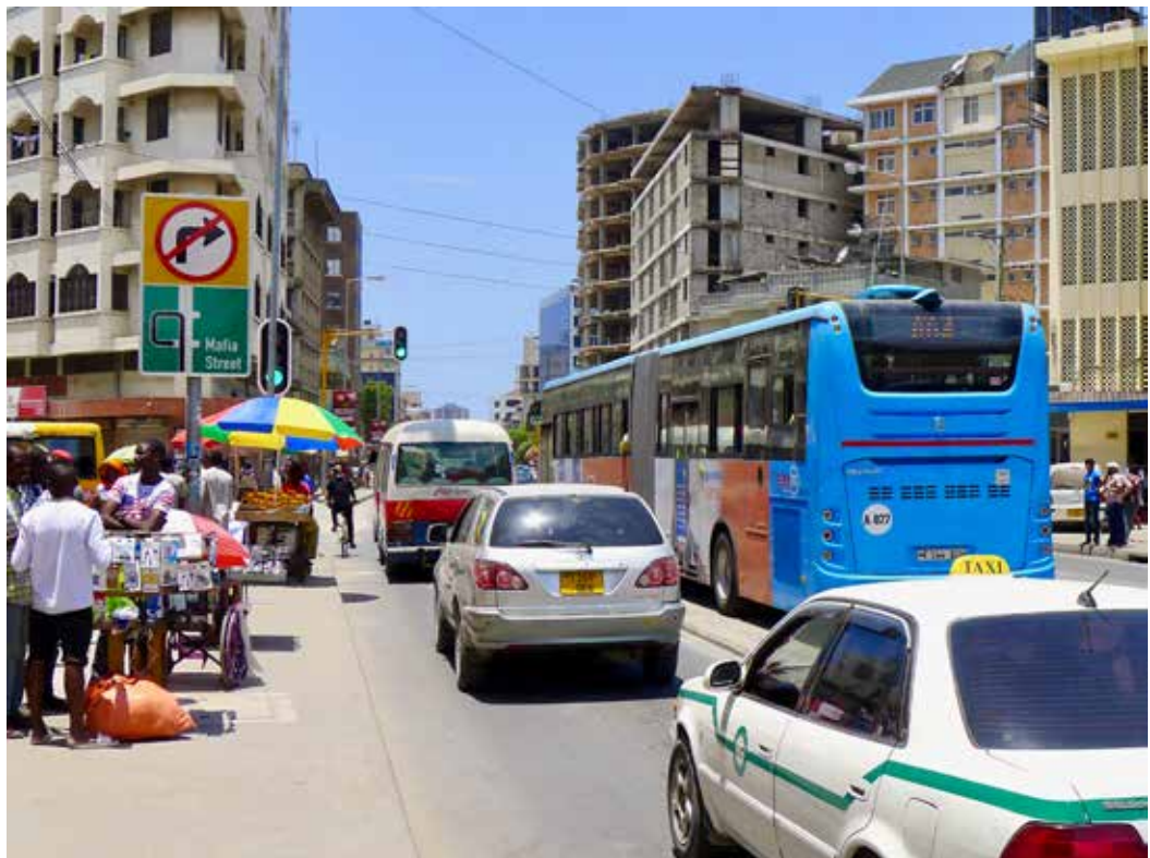
Figure 90. Signage indicating alternate mixed traffic circulation at a two-phase BRT intersection.
