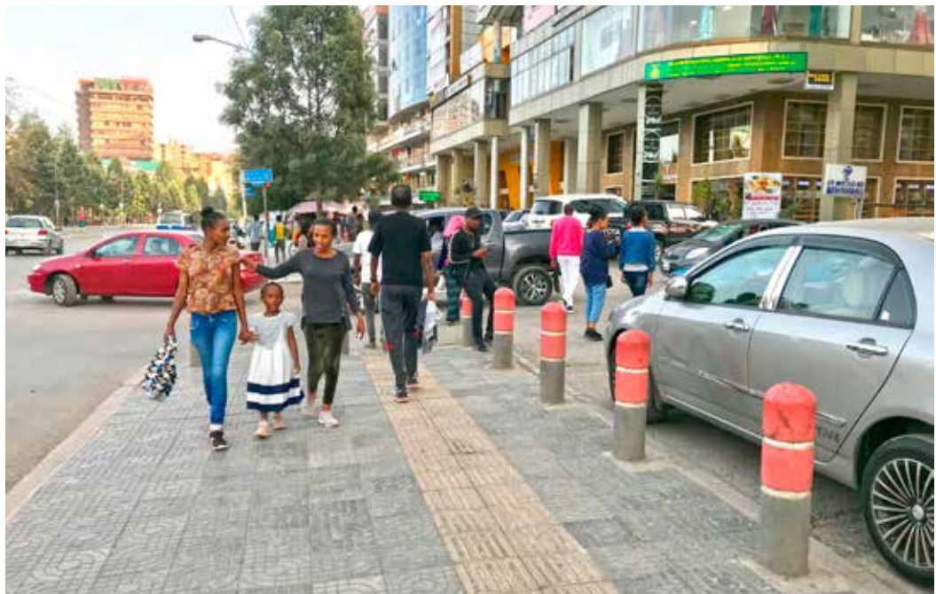
Figure 27. Bollards prevent vehicles from parking on footpaths.
