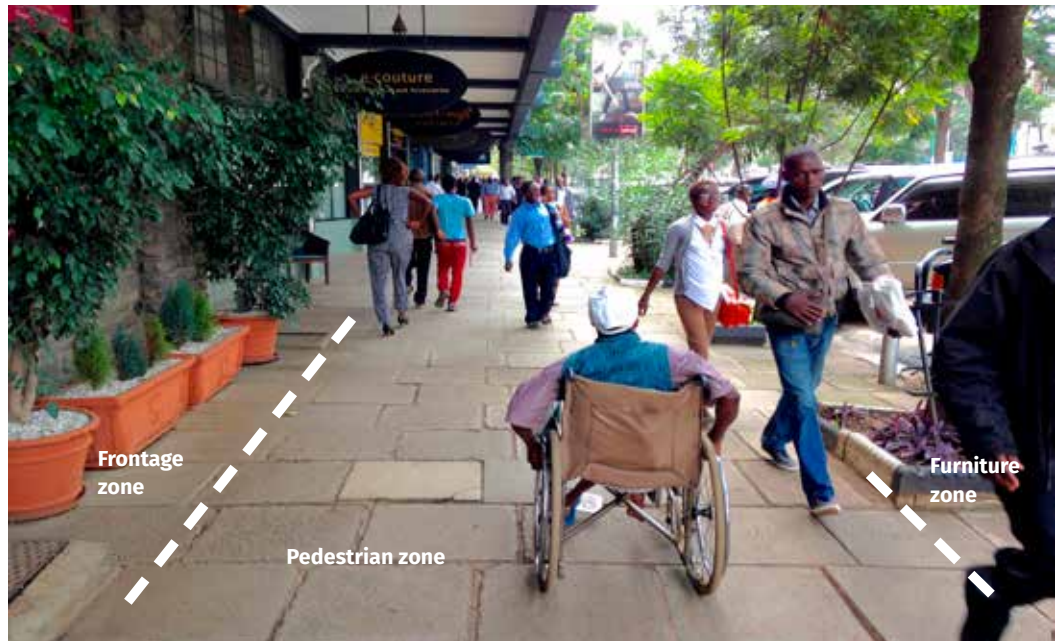
Figure 22. Footpaths designed per the zoning system provide uninterrupted walking space for pedestrians. The pedestrian zone should have at least 2 m of clear space.
